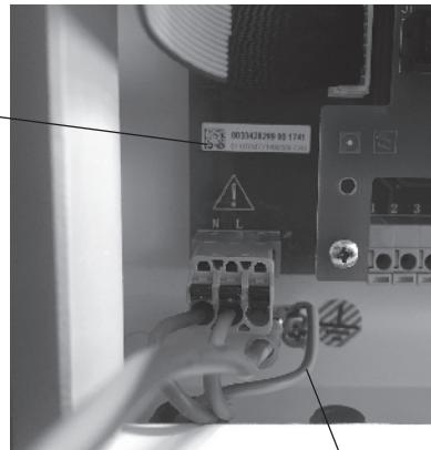
When connecting the grounding wire use the supplied blade terminals.
