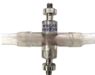
Optical Couplers Installed to Flow Cell
