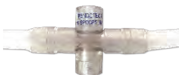
Flow Cell Installed with Tubing
