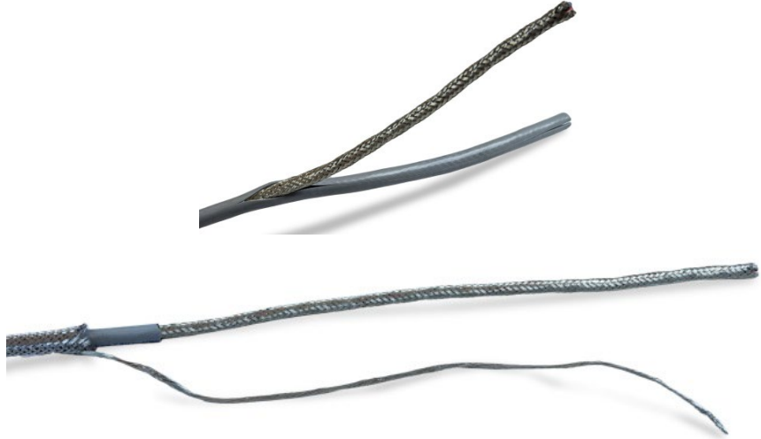
Figure A-35: Peeling the Cable Jacket away from the Inner Braided Shield
