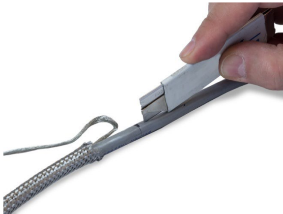
Figure A-34: Cutting Along the Cable Jacket
