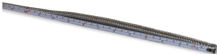
Figure A-29: Measuring the Exterior Braided Armor Before Cutting
