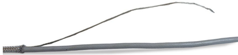
Figure A-31: Exterior Braided Armor Trimmed Back
