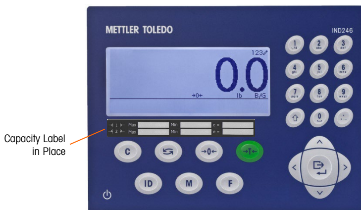
Figure A-76: Capacity Label Installed
